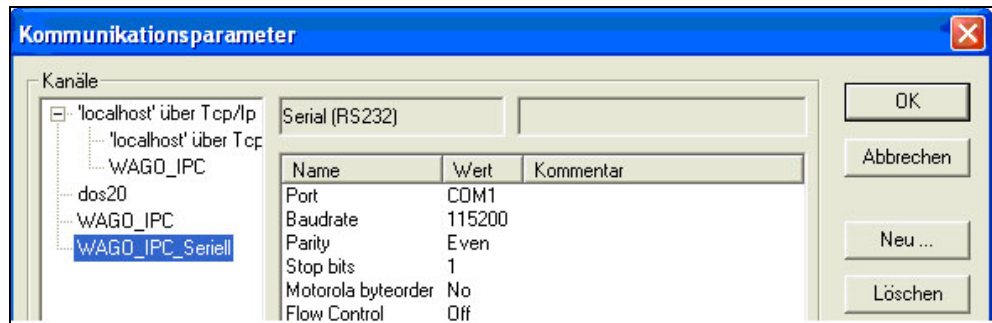
Figure 56: Creating a new communication channel (RS 232) 2
