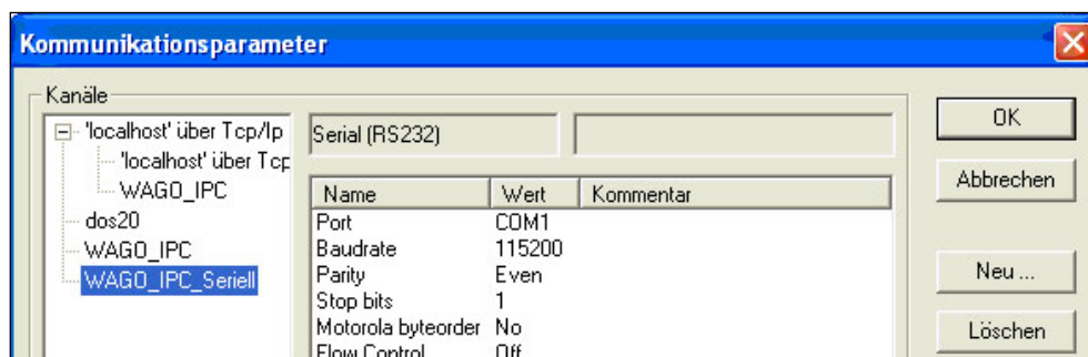
Figure 57: Creating a new communication channel (RS 232) 2
