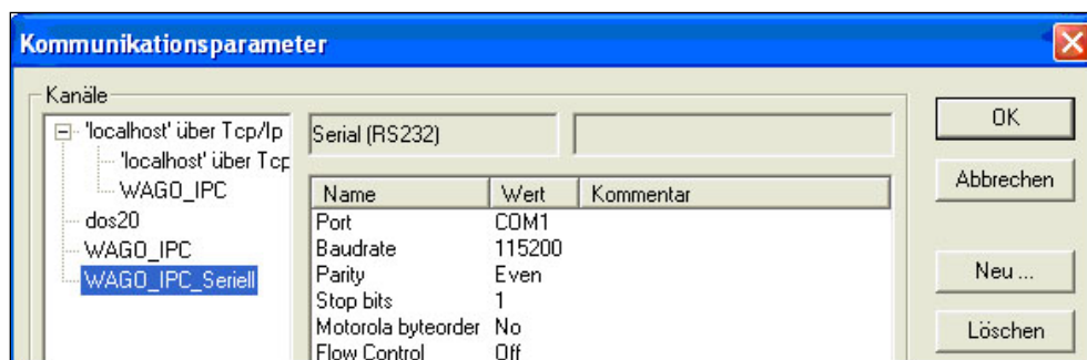
Figure 56: Creating a new communication channel (RS 232) 2
