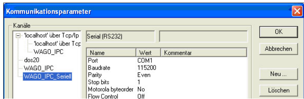
Figure 56: Creating a new communication channel (RS 232) 2
