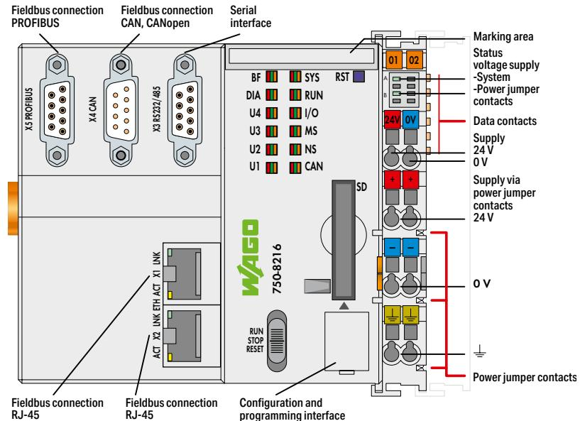
The PFC200 Controller is a compact PLC for the modular WAGO-I/O-SYSTEM. Besides network and fieldbus interfaces, the controller supports all digital, analog and specialty modules found within the 750/753 Series.
