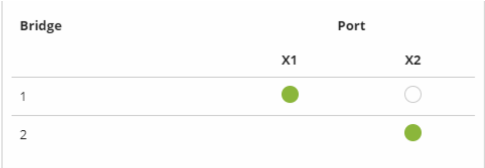
Figure 11: 2 bridges with 1/1 ports
