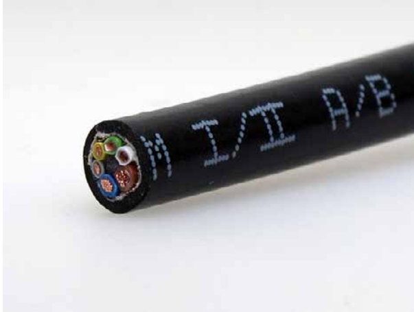
Figure 4: End of cable in as-delivered condition
