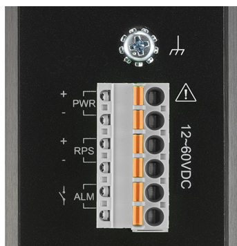
Figure 4: Power Supply Connection (PWR/RPS)
