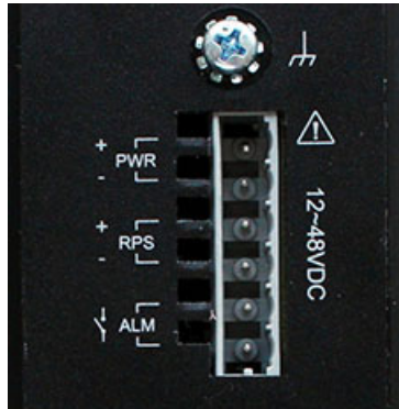
Figure 4: Power Supply (PWR/RPS)
