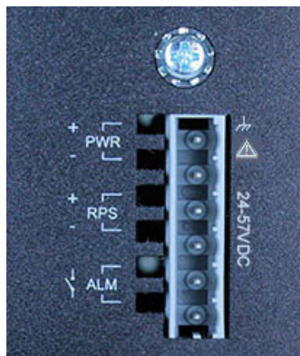
Figure 4: Power Supply (PWR/RPS)
