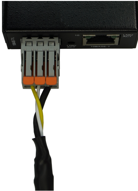
Figure 11: Data line twisting
