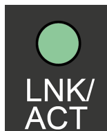
Figure 8: Status LED of the Single Pair Ethernet port
